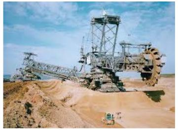
The SRs 8000, a massive bucket-wheel excavator built by German company TAKRAF, is the one of the largest moving land machines in the world. Also known as Bagger 293, it is used for strip mining brown coal in Hambach, Germany.
