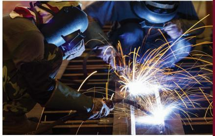
be used to remove fumes, and fume hoods, fume extractor guns, vacuum nozzles should be positioned close to the plume source to draw maximum fumes and gases. Exhaust ports should be directed away from other workers. Welding in confined spaces should not be performed without ventilation per OSHA regulations. If work practices and ventilation do not adequately reduce exposures to safe levels, respiratory protection should be used.
